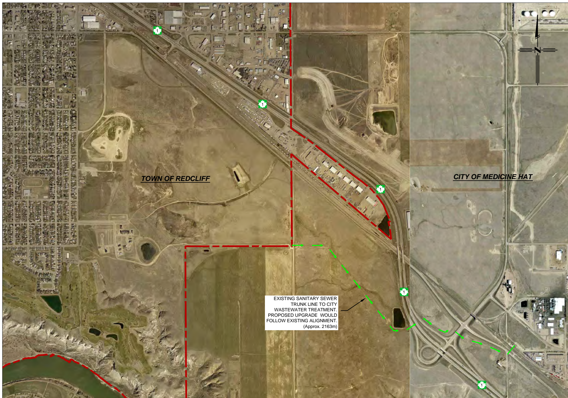
SKETCH SHOWING EXISTING AND PROPOSED SANITARY SEWER TRUNK UPGRADE
