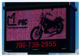
An electronic graphic display sign is defined as a sign or portion thereof that displays electronic, static images, static graphics or static pictures, with or without information, defined by a small number of matrix elements using different combinations of light-emitting diodes (LEDs), fibre optics, light bulbs or other illumination devices within the display area where the message change sequence is accomplished immediately or by means of fade, repixalization or dissolve modes.
